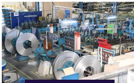
TUBE MILL OPERATION
